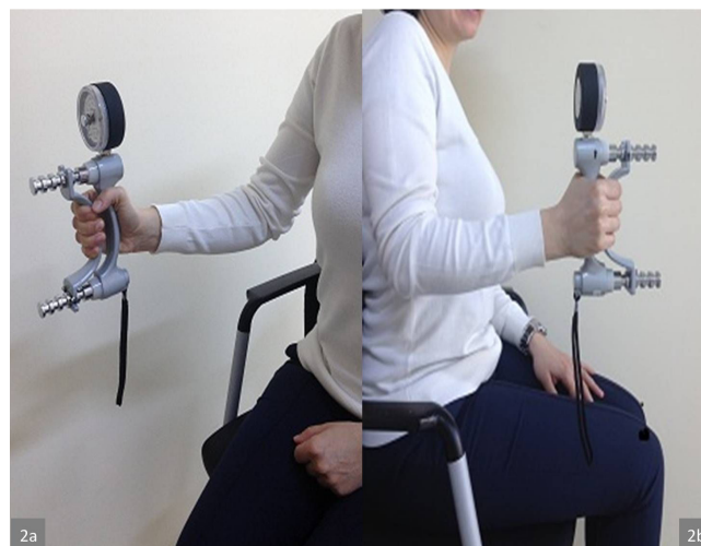
Figure 2. JAMAR hydraulic hand dynamometer measurement in a suitable position (A,B)
